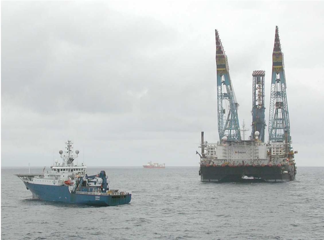
In the picture above the largest pipelay vessel in the world, Saipem's S7000 is laying a 30" pipeline in around 850m of water. The nearest ship is an ROV Survey and construction support vessel and in the background a construction vessel installing spoolpieces at the subsea template.
